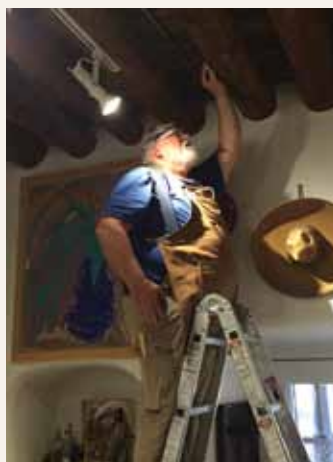
Figure 2. Tom Windes and Tom Swetnam drilling tree-ring samples from vigas in the Shop of the Rainbow Man. Photos by John Ruminer
