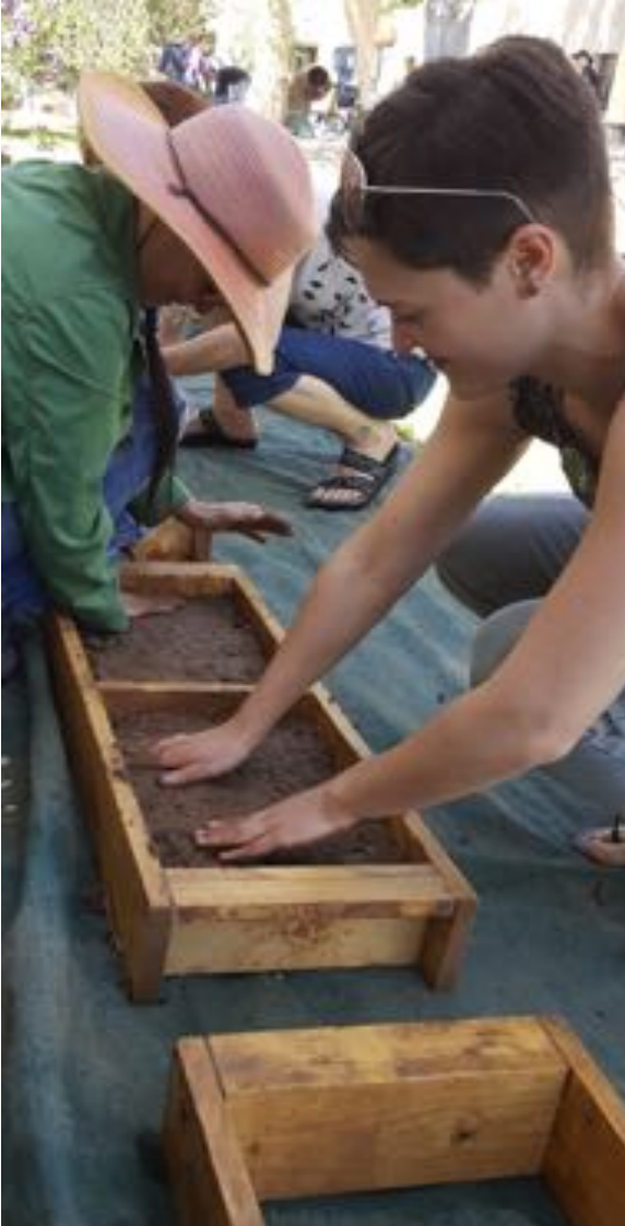
eZine cover: Melanie McWhorter, Cornerstones' intern Georgina Cantisano making adobe bricks, May 12, 2018. Instagram/historicsantafefoundation
